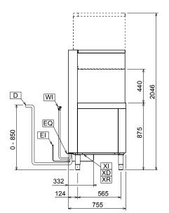
Cold Water inlet 1 (cleaning) Drain
